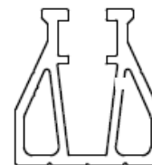
Example of neck of channel designed to accommodate an industry standard M8 square head bolt.
